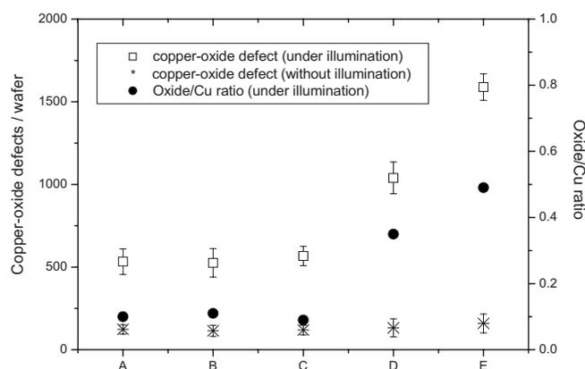
**Figure 7.** Copper-oxide defect and XPS oxide/Cu ratio for deposits with different impurity contents over 24 h after polishing under illumination.
