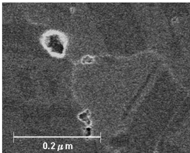
**Figure 3.** SEM image of copper-oxide defect on the copper surface after polishing 8 h (HCl dipping for 5 s to enhance grain boundaries).
