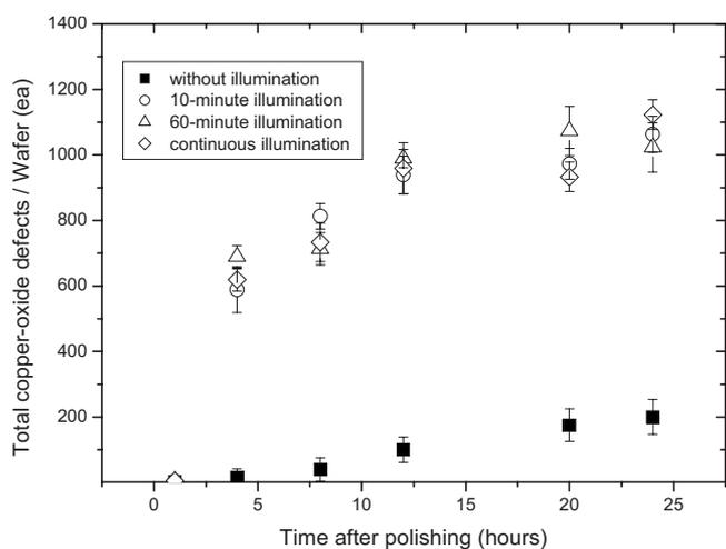
**Figure 5.** Copper-oxide defect vs time with and without illumination.
