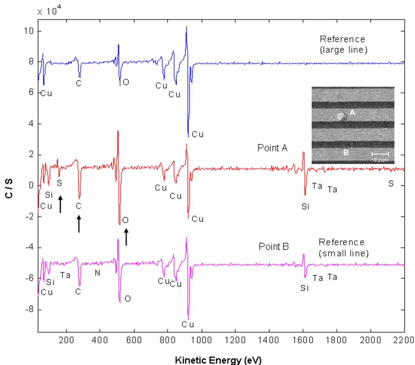
**Figure 2.** (Color online) Auger analysis for the location with and without defect on the copper-interconnect surface.
