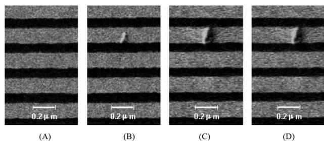
**Figure 1.** SEM images of copper-oxide defect on copper surface after polishing: (A) 2, (B) 8, (C) 24, and (D) 48 h after polishing.
