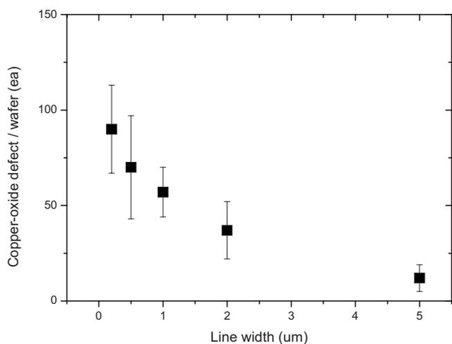
**Figure 4.** Copper-oxide defect vs line width after polishing 8 h.
