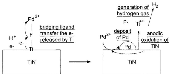
**Figure 21.** Displacement deposition of Pd: oxidation of TiN and evolution of hydrogen gas.
