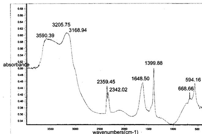
Figure 20. IR spectra of Pd activation solution after TiN reacting with  $\text{Pd}^{2+}$ .
