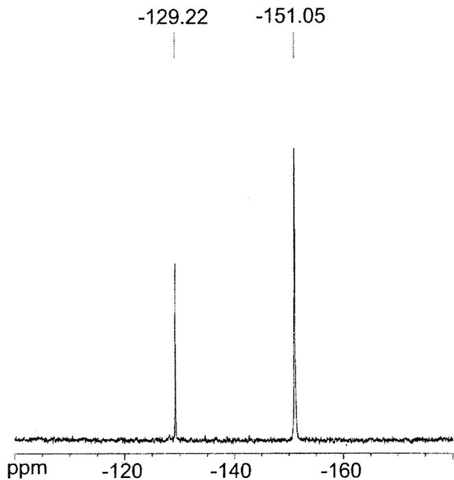
Figure 12. NMR spectra of  $F^-$  provided by NaF after the displacement reaction.
