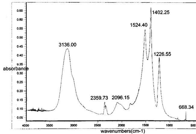
Figure 17. IR spectra before Pd displacement reaction on unsealed TaN/Si sample.
