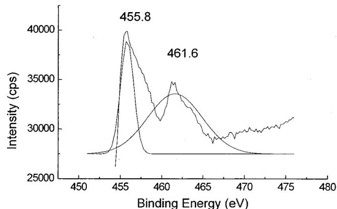
Figure 7. Oxidation-state of Ti before displacement reaction.
