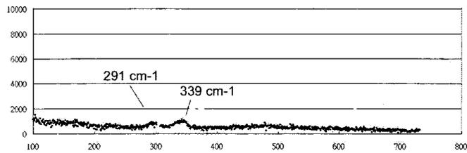
Figure 14. Raman spectra of NaF +  $PdCl_2$  solution.
