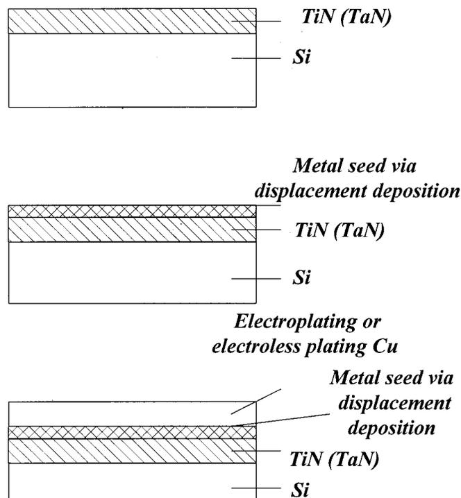
Figure 1. Process flow of Cu metallization via displacement deposition.
