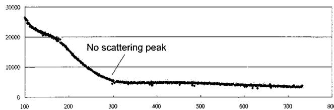
Figure 13. Raman spectra of NaF solution.
