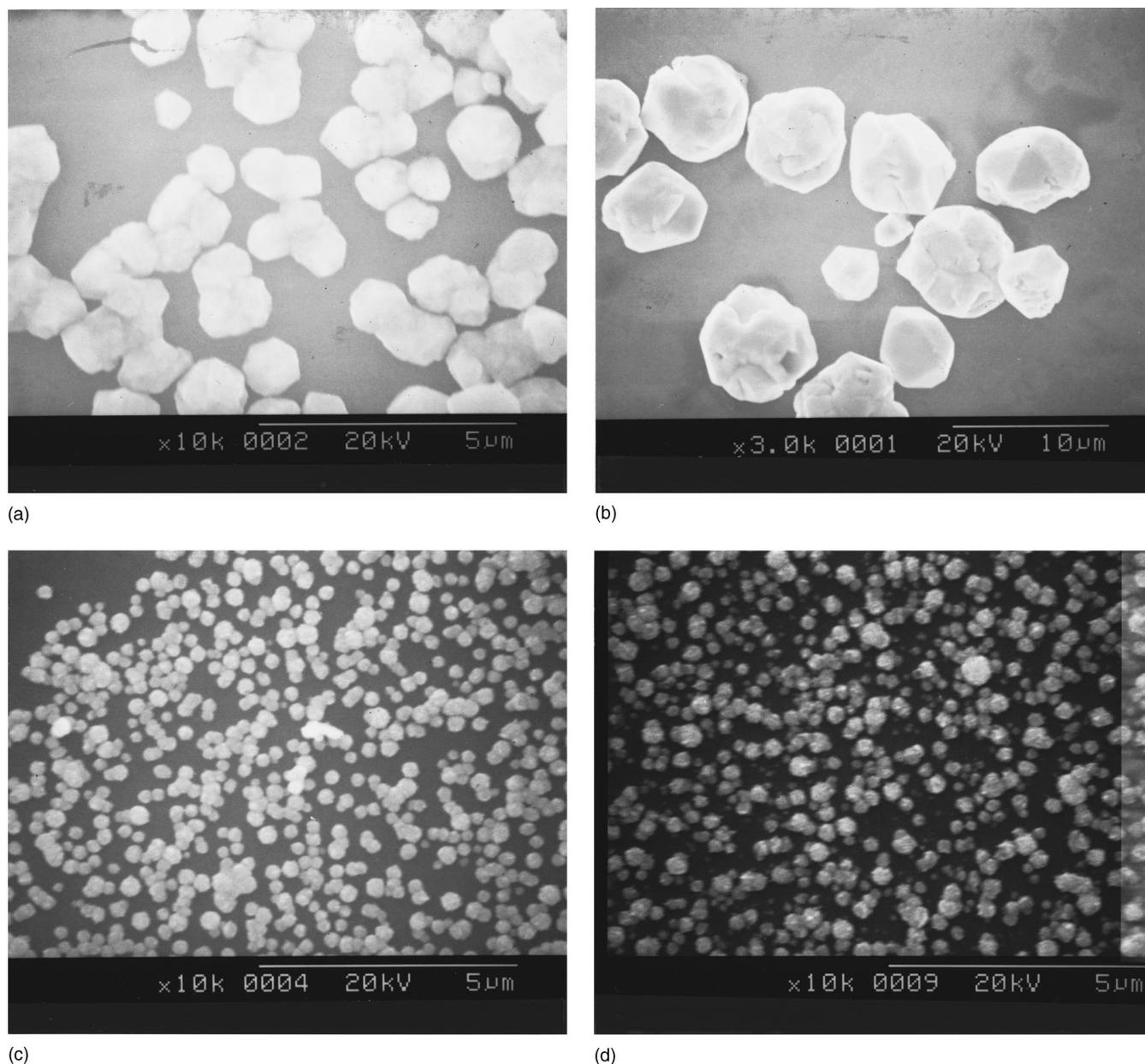
**Figure 2.** Metal deposit on the surface of nitride barrier by displacement reaction. (a) Cu deposits on TiN at a magnification of 10 k. (b) Ag deposits on TiN at a magnification of 3 k. (c) Pd deposits on TiN at a magnification of 10 k. (d) Pd deposits on TaN at a magnification of 10 k.
