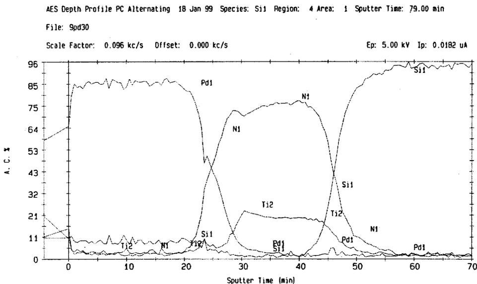
Figure 3. AES depth profile of sample after being immersed in Pd displacement solution.
