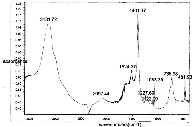
Figure 18. IR spectra after Pd displacement reaction on unsealed TaN/Si sample.
