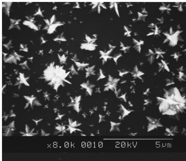
Figure 16. Needle-shape crystals found on the unsealed substrate.
