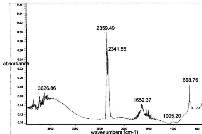
Figure 19. IR spectra of Pd activation solution before TiN reacting with  $\text{Pd}^{2+}$ .
