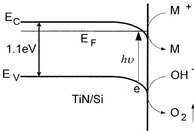
Figure 5. Second possible mechanism through photochemical reaction.
