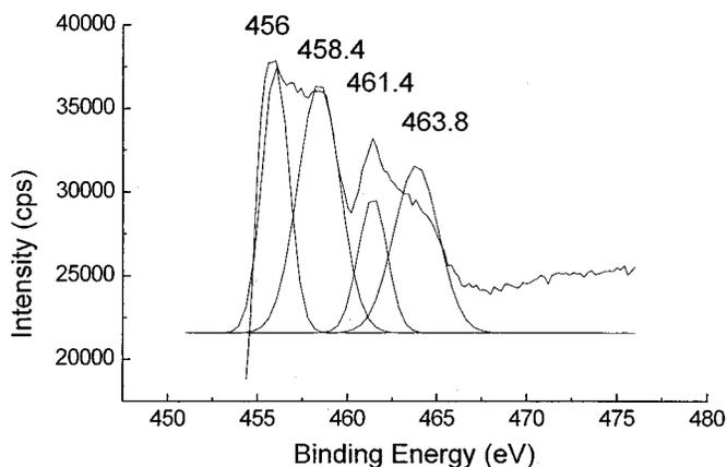
Figure 8. Oxidation-state of Ti after displacement reaction with  $\text{Pd}^{2+}$ .
