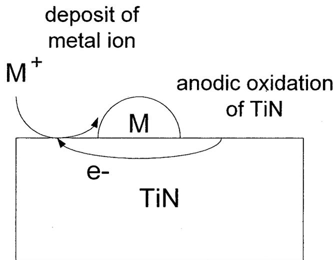
Figure 6. Anodic oxidation of TiN and cathodic reduction of metal ion in third mechanism.
