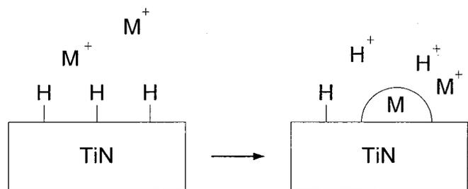
Figure 4. First possible mechanism via hydrogen-termination reaction on TiN.
