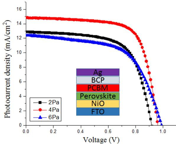
Fig. 1. J-V characteristics of inverted perovskite solar cells incorporating NiO thin films deposited under varied deposition pressure. The inset is the structure of the solar cells
