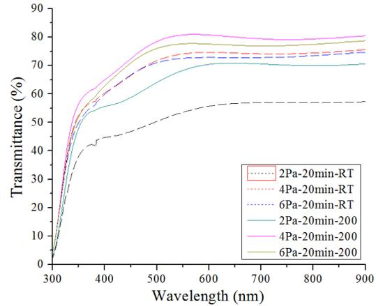
Fig. 2. Transmittance spectra of NiO thin films on ITO glasses sputtered with different deposition pressures. RT and 200 indicate the samples without and with annealing at 200 °C.
