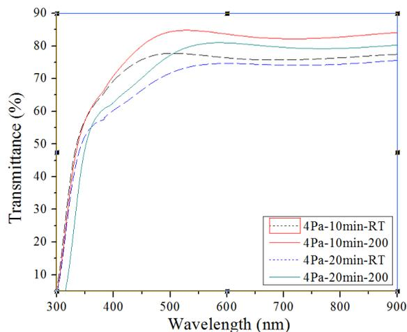
Fig. 5. Transmittance spectra for deposition-time varied NiO thin films.
