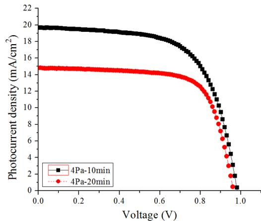
Fig. 4. Performance of inverted perovskite solar cells depending on deposition time of NiO.
