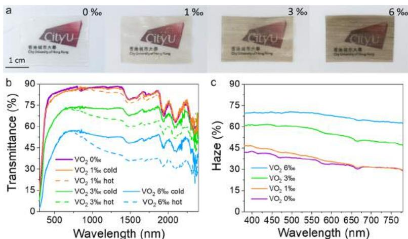
**Figure 4.** (a) Thermochromic transparent wood with different concentrations of W-doped VO<sub>2</sub> (0, 1, 3, and 6% from left to right); (b) temperature-dependent optical transmittance spectra of VO<sub>2</sub>-TTWF; and (c) optical transmittance haze of VO<sub>2</sub>-TTWF.
