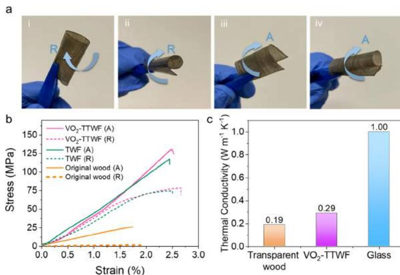
**Figure 5.** (a) VO<sub>2</sub>-TTWF was folded and rolled in A and R directions. (b) Stress–strain curves of VO<sub>2</sub>-TTWF, TWF, and original wood in A and R directions. (c) Comparison of thermal conductivity between VO<sub>2</sub>-TTWF, transparent wood, and glass.
