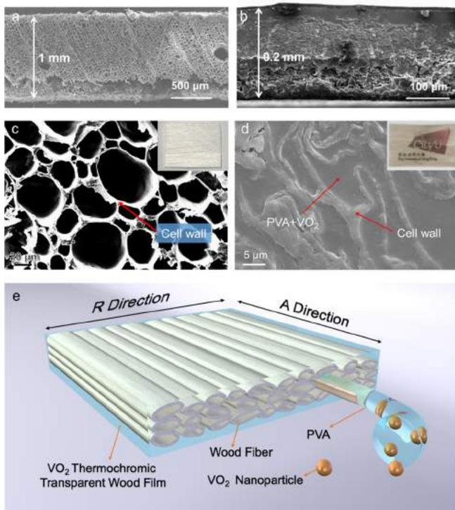
Figure 3. (a) Cross section of delignified wood. (b) Cross section of VO<sub>2</sub>-TTWF. (c) Zoomed-in SEM image of cross section of delignified wood. (d) Zoomed-in SEM image of cross section of the VO<sub>2</sub>-TTWF. Insets of (c,d) show the white wood and VO<sub>2</sub>-TTWF before and after impregnation with PVA, respectively. (e) 3D schematic of internal structure of VO<sub>2</sub>-TTWF.
