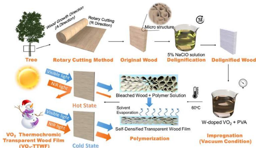
Figure 2. Fabrication process of VO<sub>2</sub>-TTWF.
