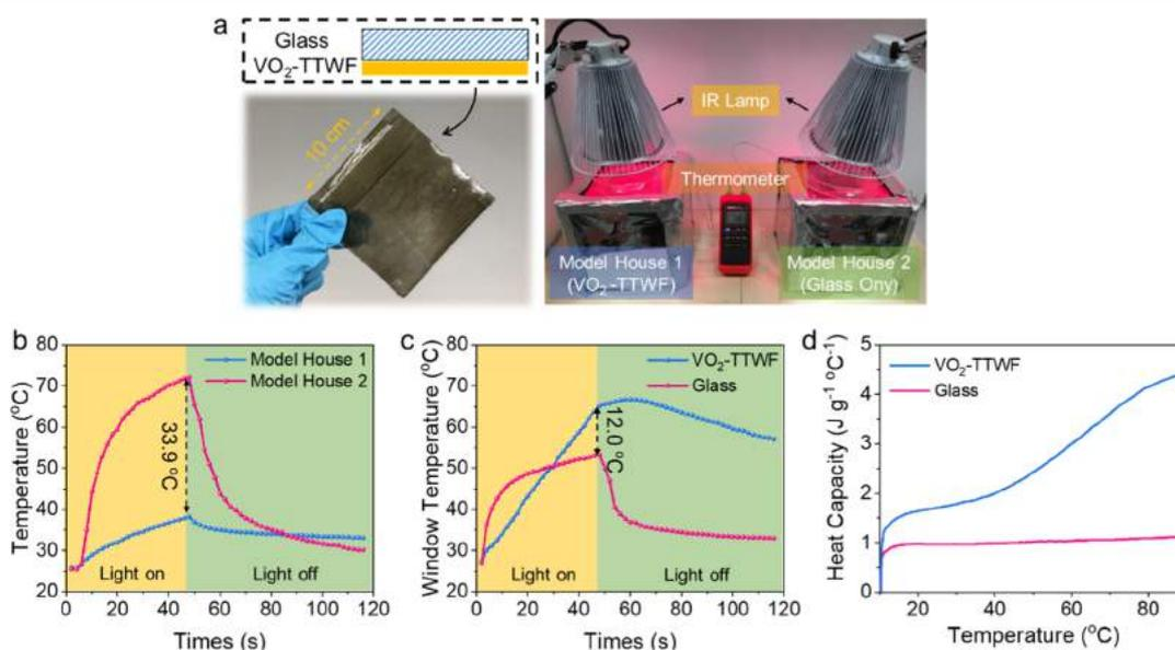
**Figure 7.** (a) Photo of VO<sub>2</sub>-TTWF pasted on the glass and the experimental set up for the model house test; (b) time-dependence of indoor air-temperature profile in model house 1 with VO<sub>2</sub>-TTWF and model house 2 with pure glass; (c) window temperature of VO<sub>2</sub>-TTWF pasted on the glass in model house 1 and the normal glass in model house 2; (d) temperature-dependent-heat capacities of VO<sub>2</sub>-TTWF and normal glass.
