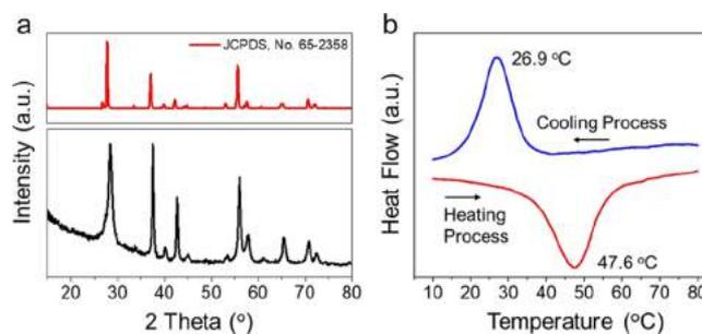
**Figure 1.** (a) XRD pattern of W-doped VO<sub>2</sub> powder and the pattern from JCPDS no. 65-2358. (b) DSC curves of W-doped VO<sub>2</sub> powder. The endothermic (red line) and exothermic (blue line) peaks indicate the transition temperature of W-doped VO<sub>2</sub> powder.
