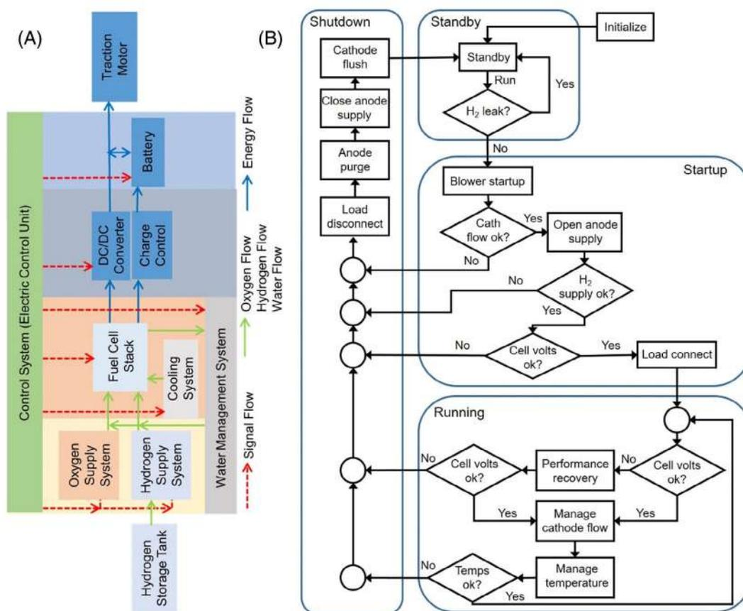
FIGURE 9 (A) Hydrogen FC hybrid system block diagram and (B) control flowchart of the FC stack [Colour figure can be viewed at [wileyonlinelibrary.com](https://onlinelibrary.wiley.com)]
