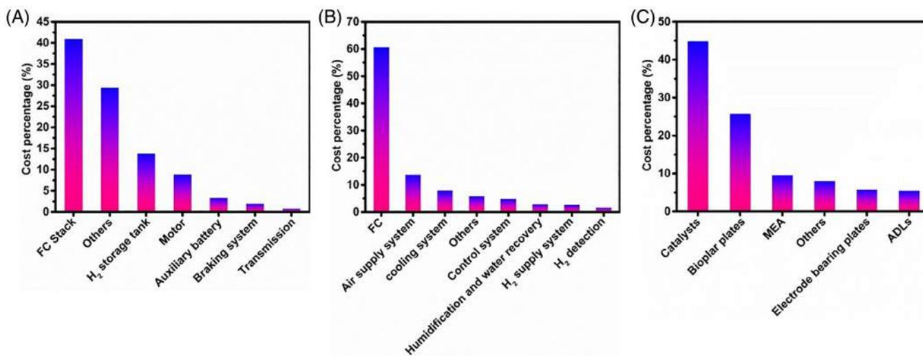
FIGURE 11 Cost breakdown of the FCHEV: (A) vehicle, (B) FC stack, and (C) FC cell<sup>186,187</sup> [Colour figure can be viewed at [wileyonlinelibrary.com](http://wileyonlinelibrary.com)]
