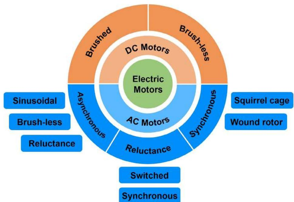
FIGURE 6 Classification of different traction motors<sup>77,125</sup> [Colour figure can be viewed at wileyonlinelibrary.com]
