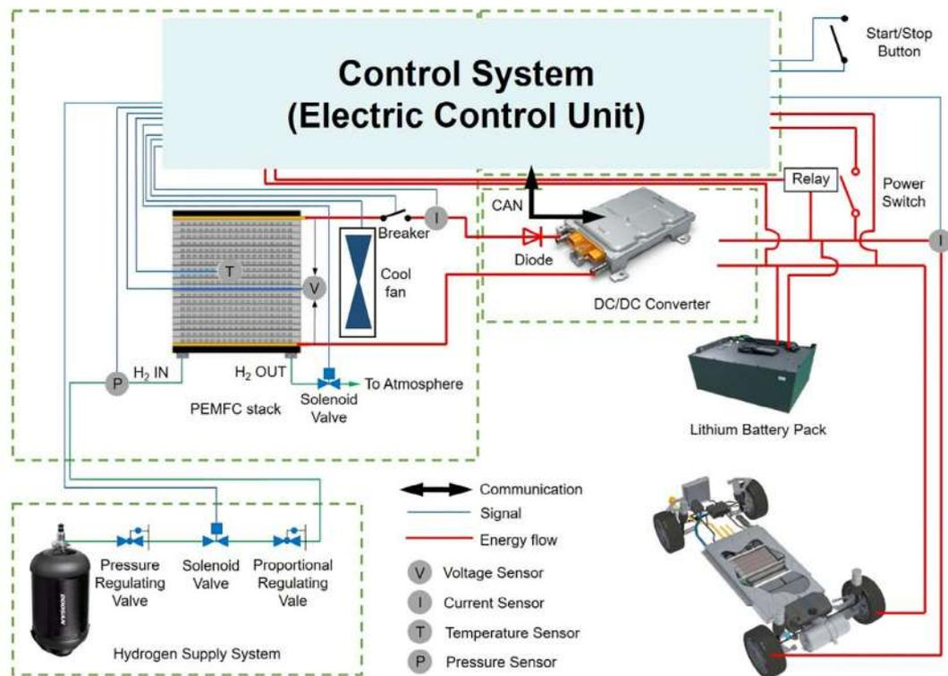
FIGURE 8 Typical optimized architecture of hydrogen FC hybrid power system [Colour figure can be viewed at wileyonlinelibrary.com]
