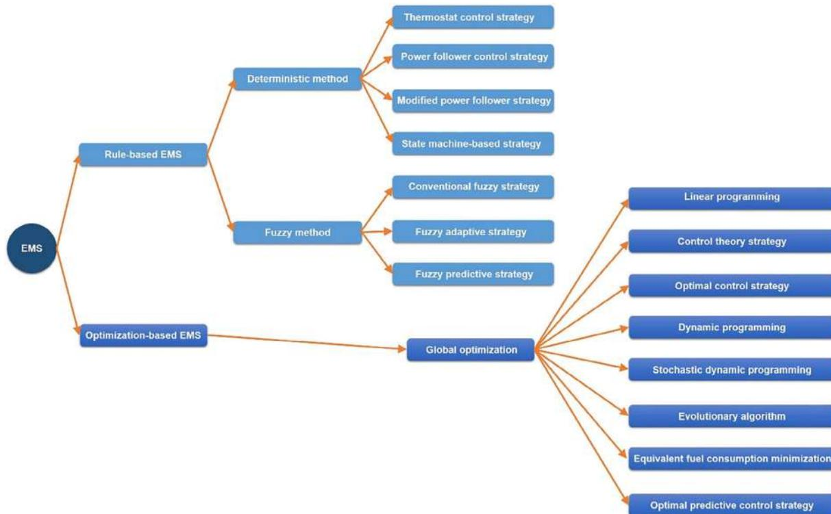
FIGURE 10 Health-conscious EMSs for FCHEVs<sup>162</sup> [Colour figure can be viewed at wileyonlinelibrary.com]
