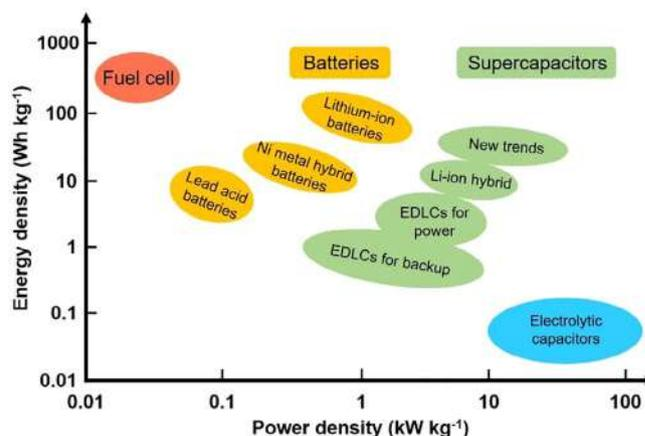
**FIGURE 1** Ragone plot of various emerging energy devices [Colour figure can be viewed at [wileyonlinelibrary.com](http://wileyonlinelibrary.com)]
