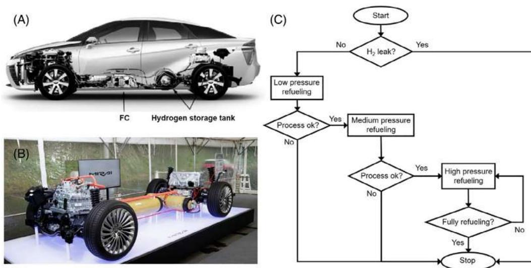
**FIGURE 12** (A) Suggested location of the hydrogen storage tank in the vehicle, (B) FC and hydrogen storage tank location in the Toyota Mirai, and (C) control flowchart of the hydrogen refueling process [Colour figure can be viewed at [wileyonlinelibrary.com](http://wileyonlinelibrary.com)]
