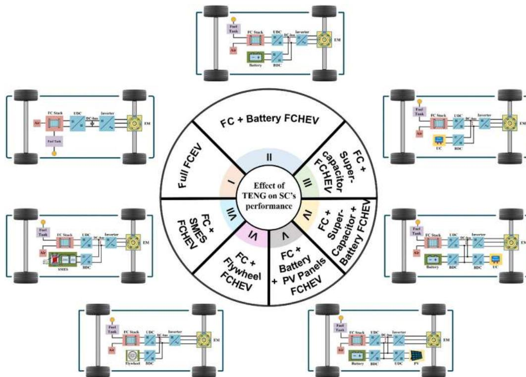
FIGURE 7 Topologies of fuel-cell hybrid electric vehicles (FCHEVs) according to the power sources<sup>77</sup> [Colour figure can be viewed at wileyonlinelibrary.com]
