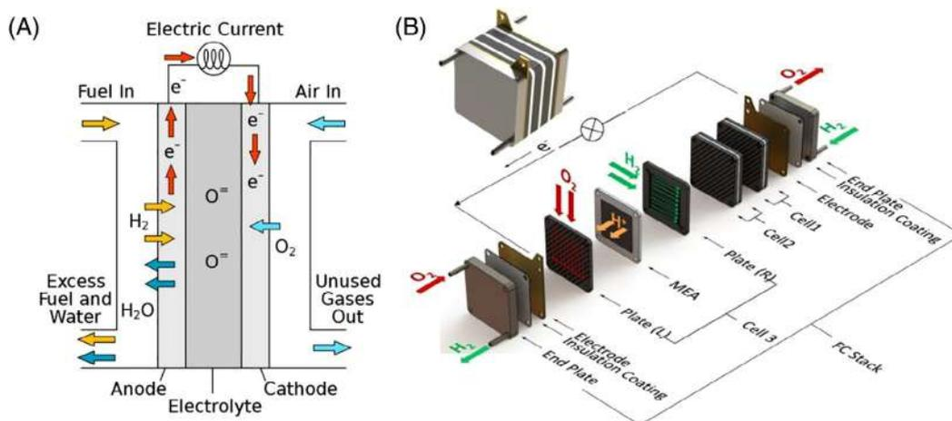
FIGURE 3 Concept of (A) a single fuel cell (FC) and (B) proton exchange membrane fuel cell (PEMFC) stack.<sup>53,54</sup> Copyright © 2021 Wipedia and 2017 Elsevier [Colour figure can be viewed at wileyonlinelibrary.com]
