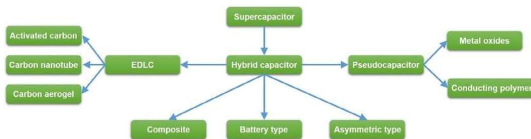
FIGURE 5 Classification of supercapacitors [Colour figure can be viewed at wileyonlinelibrary.com]
