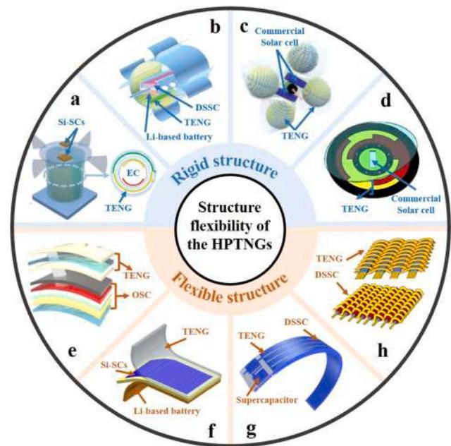
**Fig. 3.** Structural flexibility of HPTNGs: (a) Schematic of the hybrid energy cell. (b) Schematic of the self-powered lantern. (d) Schematic of self-powered control disk. (e) Schematic of the flexible hybrid cell. (f) Schematic of the flexible hybrid energy harvesting device. (g) Schematic of the flexible hybrid power bracelet.
