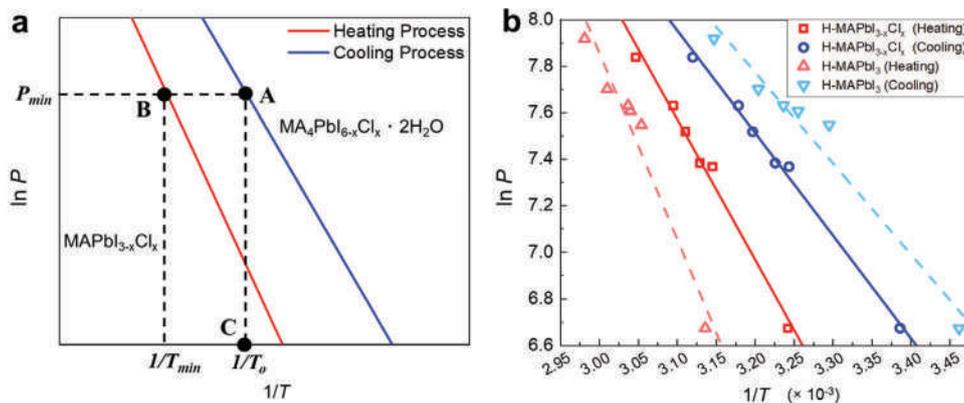
**Figure 4.** a) Pressure–temperature dependent transition model of thermochromic perovskite in the Clausius–Clapeyron diagram. b) Measurement points upon transition temperature and water vapor pressure of H-MAPbI<sub>3-x</sub>Cl<sub>x</sub> and H-MAPbI<sub>3</sub> thermochromic perovskites as well as the fitted curve in the Clausius–Clapeyron diagram (solid and dash lines, respectively).
