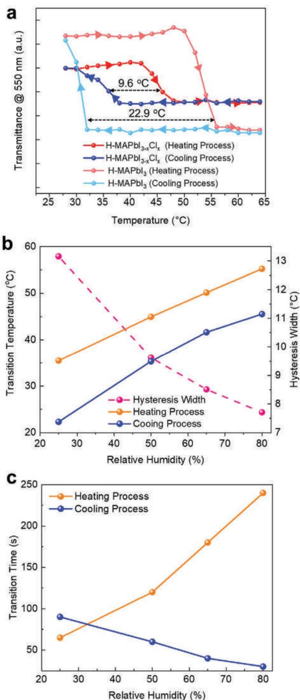
**Figure 3.** a) The temperature-dependent thermochromic hysteresis loops of the H-MAPbI<sub>3-x</sub>Cl<sub>x</sub> and H-MAPbI<sub>3</sub> TPSWs upon heating and cooling processes (optical transmittance at 550 nm as a function of temperature). b) Effect of RH on the  $T_c$  and  $\Delta T_c$  of the H-MAPbI<sub>3-x</sub>Cl<sub>x</sub> TPSW. c) Effect of RH on the  $t_c$  of the H-MAPbI<sub>3-x</sub>Cl<sub>x</sub> TPSW upon heating and cooling processes.
