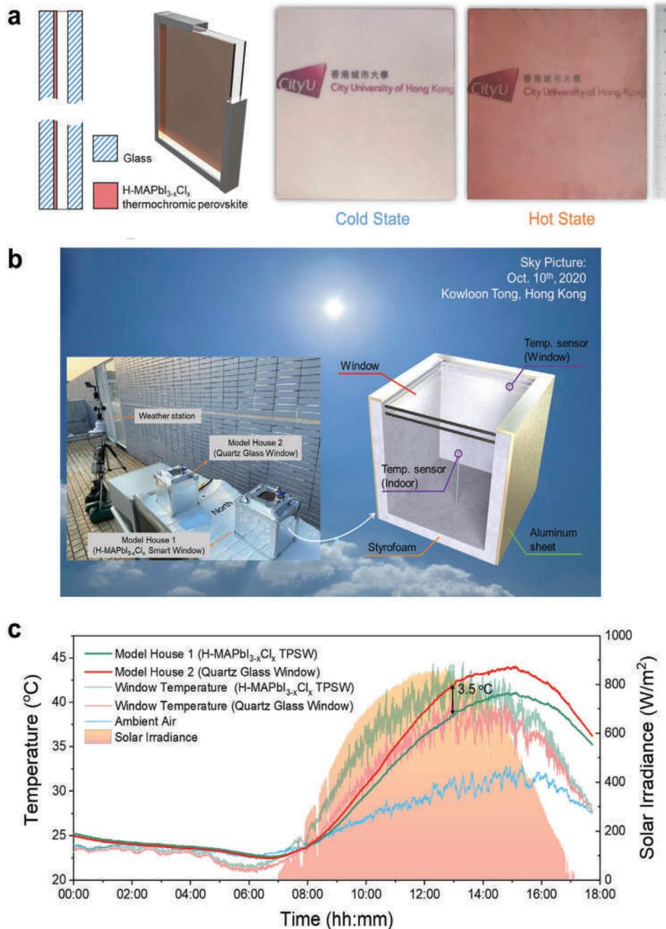
**Figure 6.** a) Schematics of the double-glazed H-MAPbI<sub>3-x</sub>Cl<sub>x</sub> TPSW and the 9 cm × 9 cm glass at the cold and hot states for the model house field test. b) Scheme of model house field test set up. c) 18 h temperature curve for the model house field test on the 10th October, 2020 in Hong Kong.
