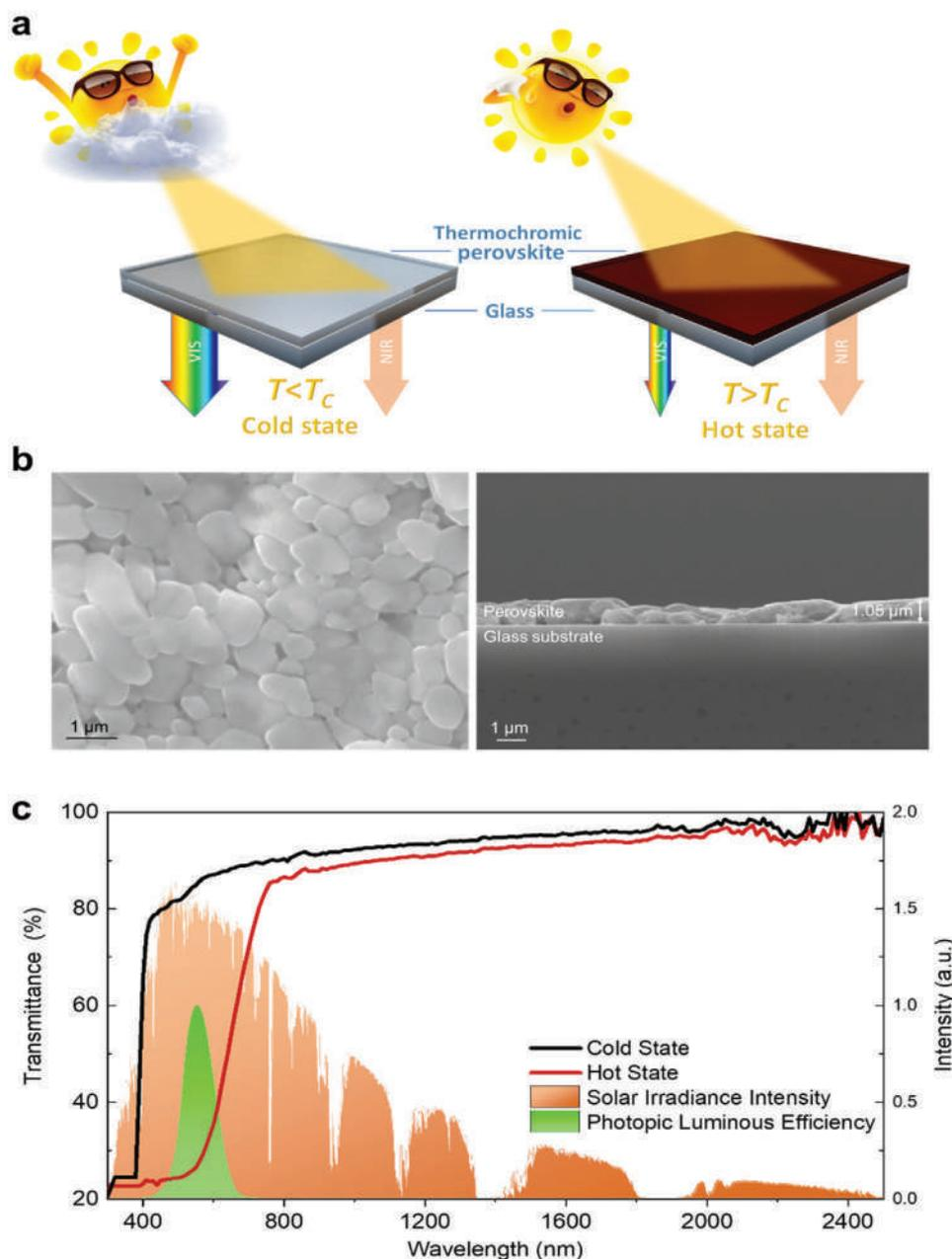
**Figure 2.** a) Working principle of H-MAPbI<sub>3-x</sub>Cl<sub>x</sub> TPSW. b) SEM image of H-MAPbI<sub>3-x</sub>Cl<sub>x</sub> thermochromic perovskite thin film. c) Transmittance spectrum of H-MAPbI<sub>3-x</sub>Cl<sub>x</sub> TPSW at the cold and hot states.
