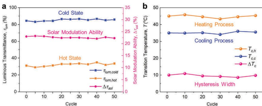
**Figure 5.** a) Optical performance ( $\tau_{lum,hot}$ ,  $\tau_{lum,cold}$ , and  $\Delta\tau_{sol}$ ) of the H-MAPbI<sub>3-x</sub>Cl<sub>x</sub> TPSW after 50 cycles. b) Transition properties ( $T_{c,h}$ ,  $T_{c,c}$ , and  $\Delta T_c$ ) of the H-MAPbI<sub>3-x</sub>Cl<sub>x</sub> TPSW after 50 cycles.
