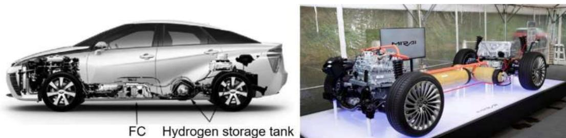
Fig. 18. Schematic of FC and hydrogen storage tank in the Toyota Mirai.
