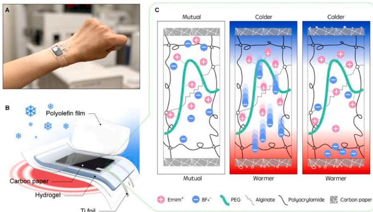
**Fig. 1.** Pam-alginate/EmimBF<sub>4</sub>/PEG. (A) Digital image of a thermoelectric wristband made of Pam-alginate/EmimBF<sub>4</sub>/PEG. (B) System of Pam-alginate/EmimBF<sub>4</sub>/PEG consisting of Pam-alginate hydrogel electrolyte including EmimBF<sub>4</sub> IL and PEG, nanoporous CP electrodes, Ti conductors and polyolefin wrap. (C) Schematic illustration of generating thermovoltage in Pam-alginate/EmimBF<sub>4</sub>/PEG.
