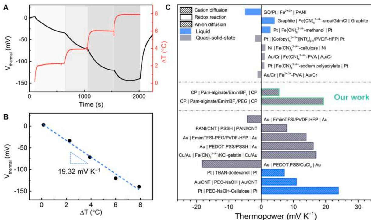
**Fig. 2.** Thermopower characterization. (A) Thermovoltage versus temperature gradient plot. (B) Thermopower of Pam-alginate/EmimBF<sub>4</sub>/PEG. (C) Comparison of thermopower for Pam-alginate/EmimBF<sub>4</sub>/PEG with some of the best reported TECs and i-TEs (see Appendix). The thermoelectric systems inclusive of electrolytes and electrodes are presented.
