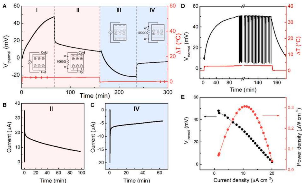
**Fig. 4.** Power generation in Pam-alginate/EmimBF<sub>4</sub>/PEG. (A) Four-stage charging-discharging behaviors of Pam-alginate/EmimBF<sub>4</sub>/PEG. Inserts present corresponding electron flow. (B) and (C) Current plots in electrical charging (stage II), and discharging (stage IV), respectively. (D) Thermovoltage profile in quasicontinuous charging/discharging process for 30 cycles. (E) Power density (red) and thermovoltage (black) of the first cycle in D.
